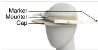
Figure 3, Moulder for infrared reflective markers that has six mounting holes to be set markers in various position combinations.
