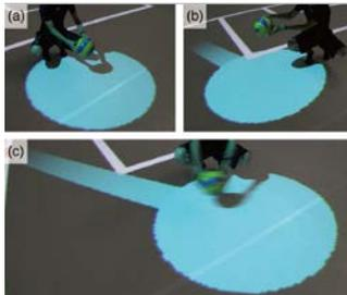
Figure 6, Predicted path of a ball (a) stopping, (b) moving slowly, (c) moving quickly, the length of predicted path scales linearly with the velocity.
