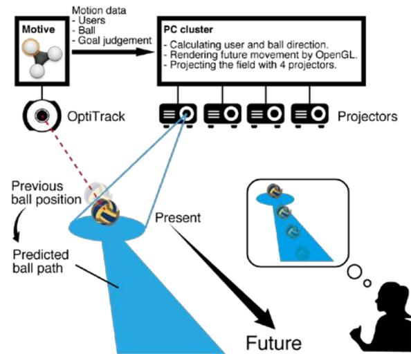
Figure 4: System Configuration of Sport Support System that have 22 motion capture cameras for tracking the ball and users at very high accuracy less than 1mm and four FHD projectors for projecting ball path and players position.
