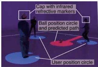
Figure 5: Implementation results for Sports Support System for soccer, the proposed system can track six of players and the ball and visualize those positions and predicted direction.
