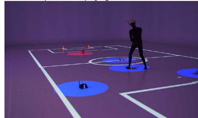
**Figure 1:** Overview of Sport Support System, that is a projection-based augmented reality system for supporting ball game training, provides the trajectory and velocity of the ball and players on a marker projection on the floor.
